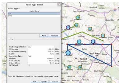
1. The **RFview™** tool supports the creation of dynamic multipath scenarios with real and virtual radios. An API allows the user to import specific channel modeling tools or recorded field test data.
