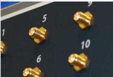
Emulation hardware with RF front ends that allows real radio nodes to send their RF signals over an emulated channel without any modification to the radios.
