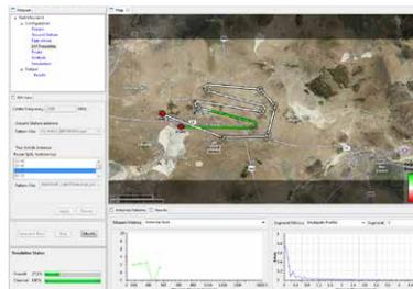
Modeling of time-varying channel impulse responses within the emulation hardware, with channel properties based on mobility models receiving input from an interactive Graphical User Interface (GUI).
