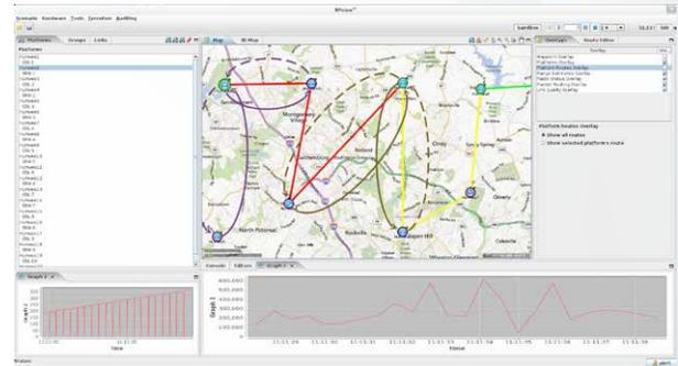
**RFnest™** Testing of three wireless networks at the same time; two nodes transmitting bulk data at 900 MHz frequency band, video communication between two nodes in 2.4 GHz band, two real nodes and 7 virtual nodes forming a multi-hop wireless network transmitting bulk data at 2.4 GHz frequency band.
